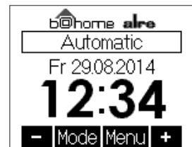
Display screen after assignment for the control of individual rooms
