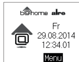
Display screen after assignment for central control
